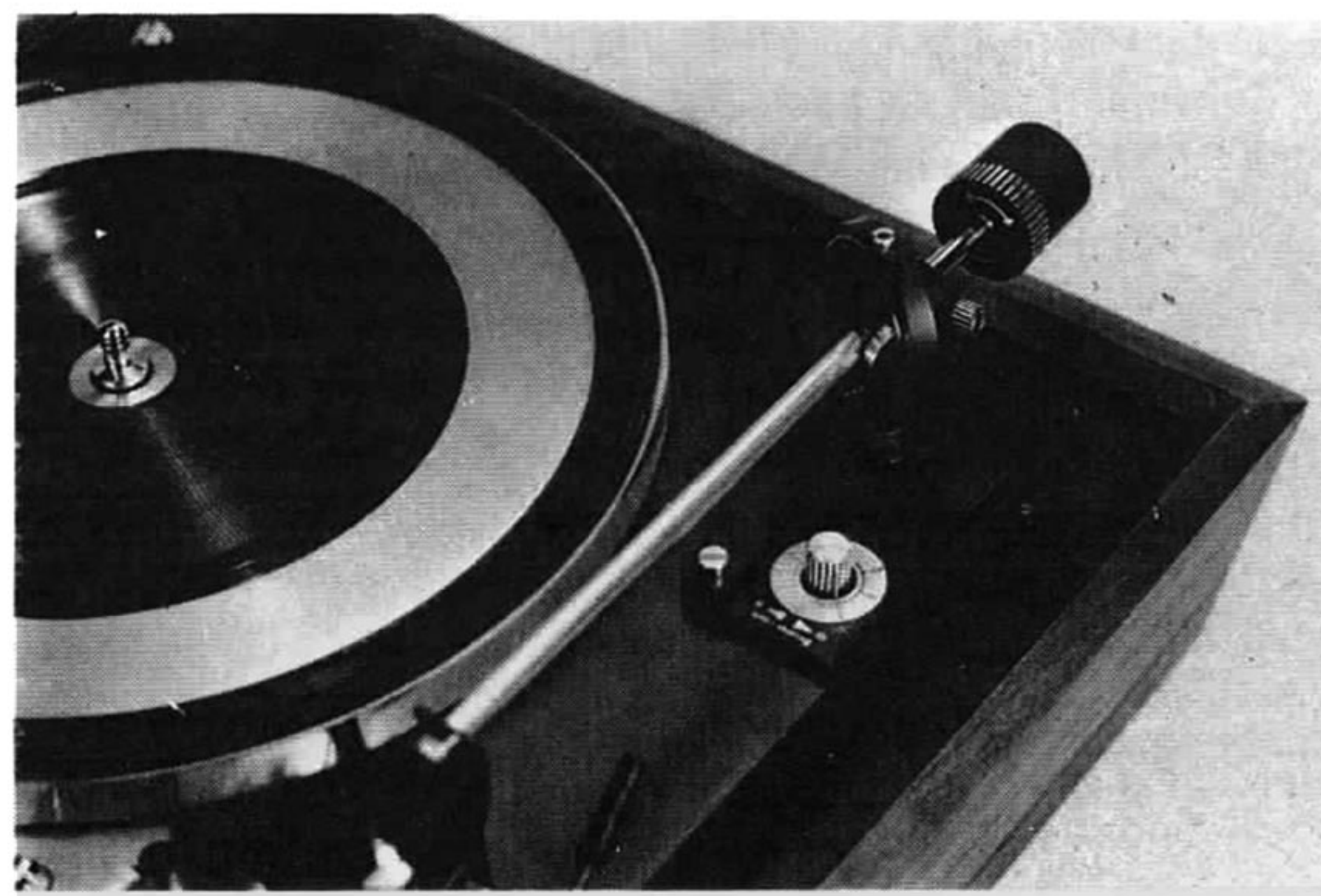
Fig. 1 —Most adjustments are found near the arm mounting—coarse and fine counterbalance, stylus force, anti-skating, and tonearm cueing height. Note record spindle for single-play use—it rotates with the platter to avoid wearing the center hole and to ensure concentricity.
